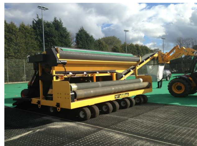
Automatic carpet lifting and rolling operation
